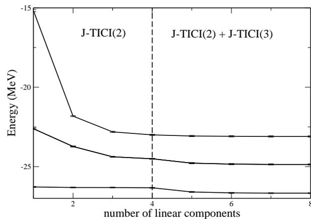
Figure 5.25: The ground-state energy for the J-TICI(2)+J-TICI(3) calculation of  ${}^6\text{He}$  as a result of the total number of linear components used. The first four components (left-hand side of the vertical broken line) include only two-body correlations while the remaining components (right-hand side of the broken line) include the added three-body correlations. The results were obtained for the S3 interaction.
